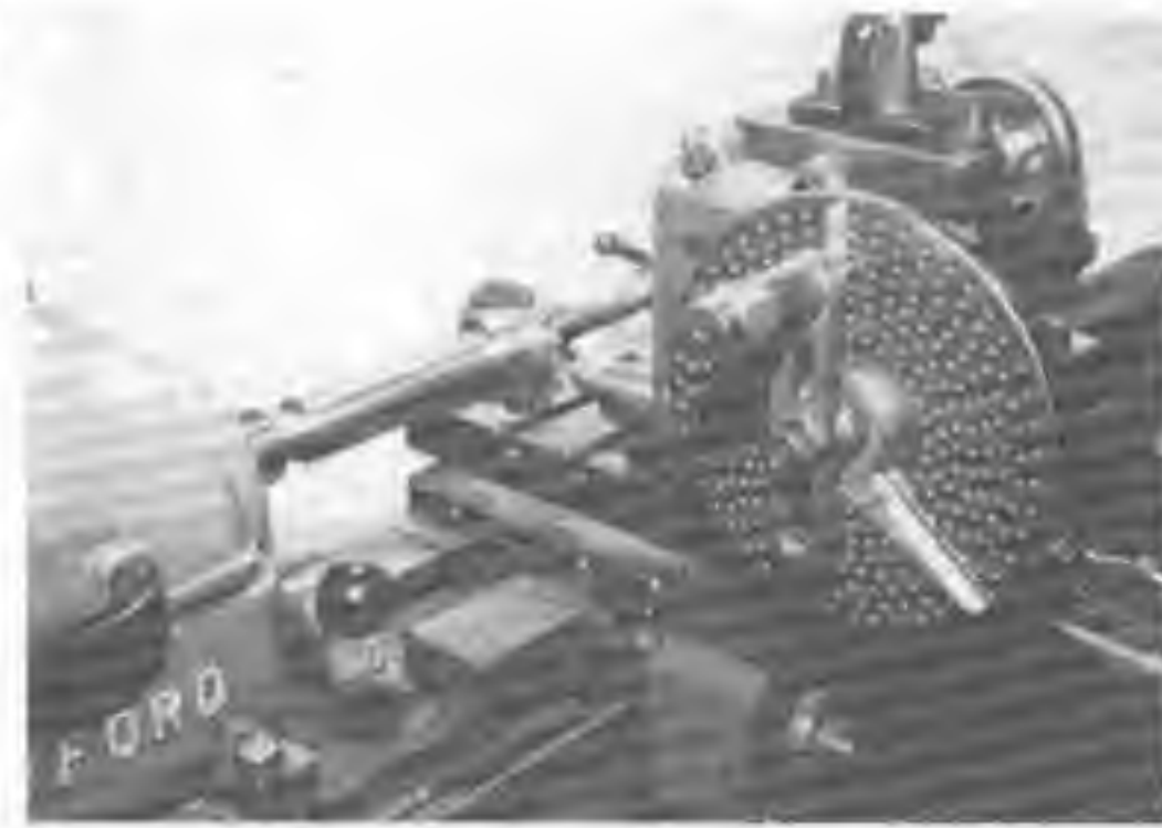
Fig. 58 Positioning the cutter by using a lathe centre as a temporary arbor replacement.
